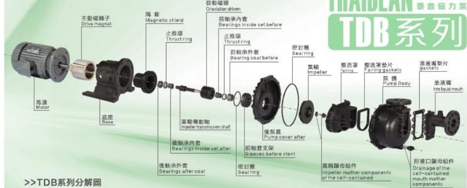
>> TDB系列分解圖 TDB series decomposition figure
